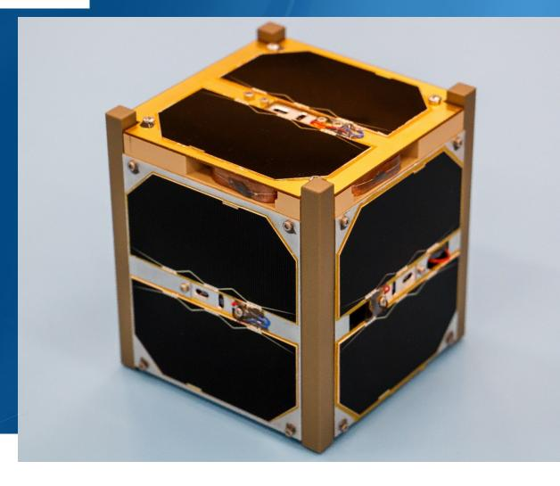
A "standard 1U" CubeSat has a volume of one liter - 10 cm cube and a mass of 1 kg, orbiting at 300-600 km circular orbit, 1W transmitter on 145 or 435 MHz amateursatellite service band. It's used for academic education, research and technology validation applications but also for complex science and governmental use
